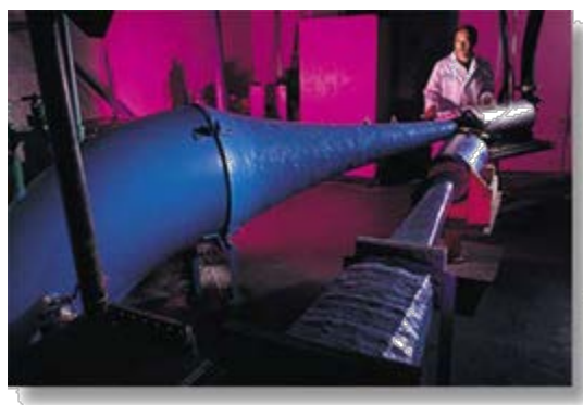
Wyle's 1500-cubic foot (42.5m 3 ), high-intensity acoustic facility Showing the WAS 3000, parallel test section and reverberant chamber
