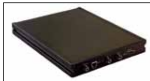
Rear panel provides a 100Base-T female RJ45 Ethernet connection, a LIMO five-pin Spider-NAS port, an RS-485 serial port, a DB25 Digital I/O connector and a 15 VDC (±10 %, 10 watt) power input connector.
