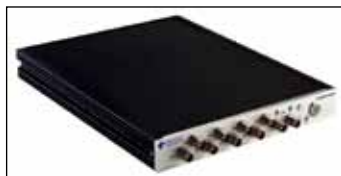
Spider-80X module accepts eight analog signals and two tachometer signals through front panel BNC connectors; it provides a power switch and status LEDs (power, run/stop, flash memory capacity, LAN communication).
