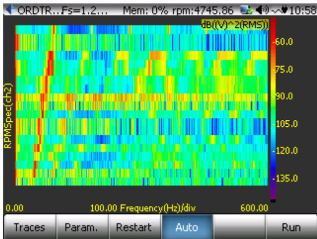
■ Figure 31 Color map of an RPM spectrum.
