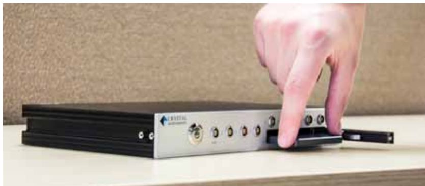
The Spider-NAS features eight dedicated high-speed data buses and a removable 250 GB serial ATA (SATA) Solid State Disk (SSD).
