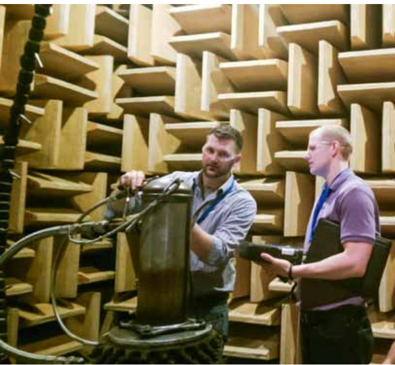
The CoCo-80 combines with a microphone to take measurements inside an anechoic chamber
